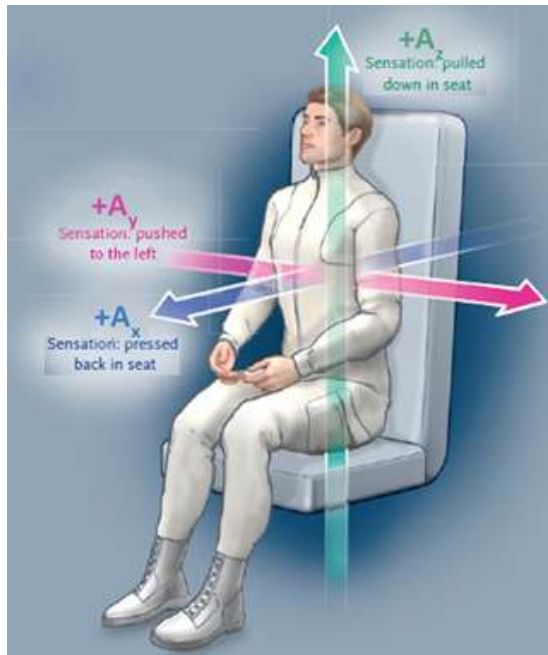
Figure 6.5-1—Common XYZ Coordinate Frame for Translational Acceleration
