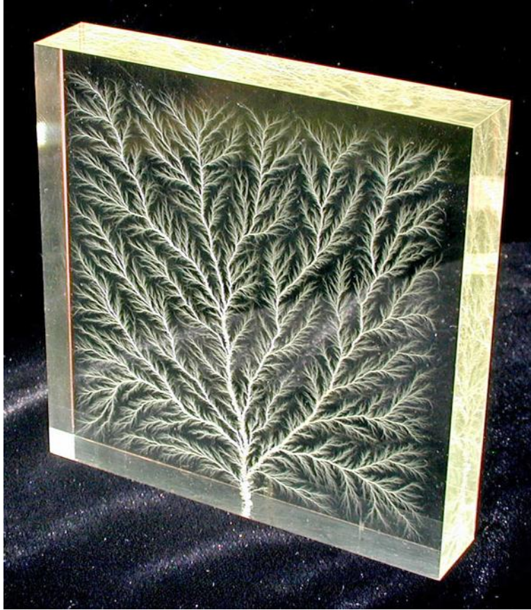
Figure 46—Electrical Treeing in Plexiglass (author: Bert Hickman)
