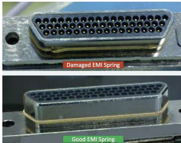
Figure 2 - Damaged EMI Spring (above) and Intact EMI Spring (below)
