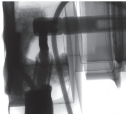
Figure 3 - X-Ray Image of Internal Kinked Conductor
