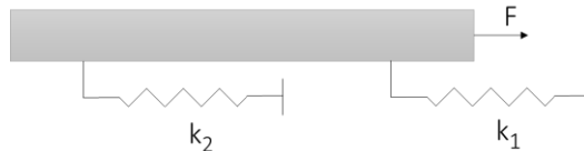
Figure 22a—Simplified Two-Bolt Plasticity Model
