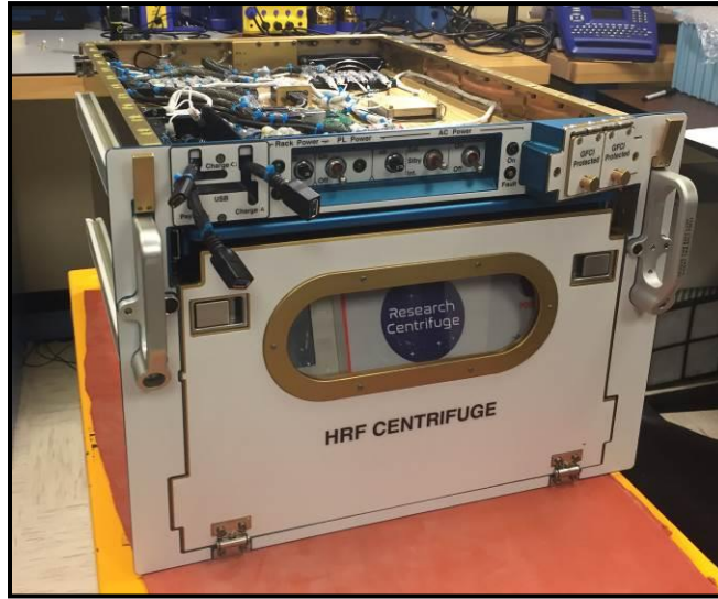
Figure 6.1-2—Picture of 8PU Locker with Centrifuge Inside
