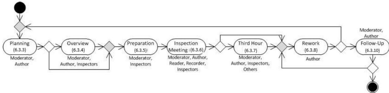
Figure 1. Inspection Process
