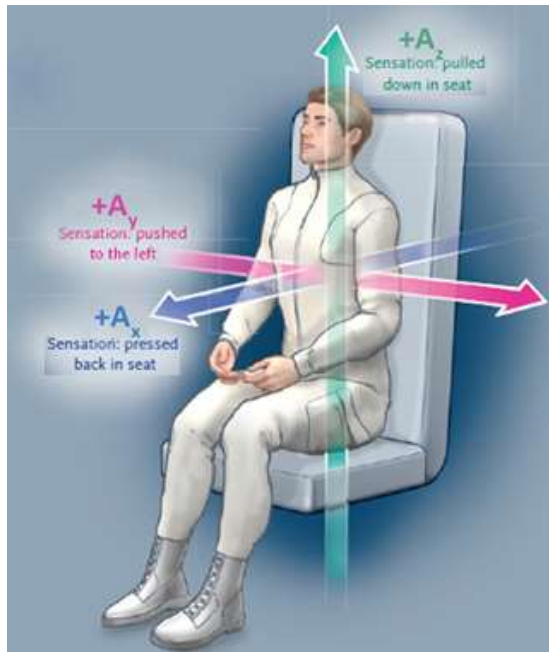
Figure 6.5-1—Common XYZ Coordinate Frame for Translational Acceleration
