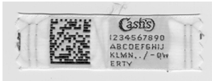
Figure 27—Cloth Label Produced Using Fabric-Weaving Technique
