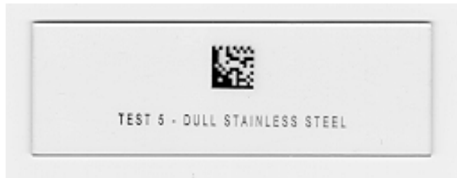
Figure 37—Stainless Steel Marking Applied to Glass Slide Using LIVD Process
