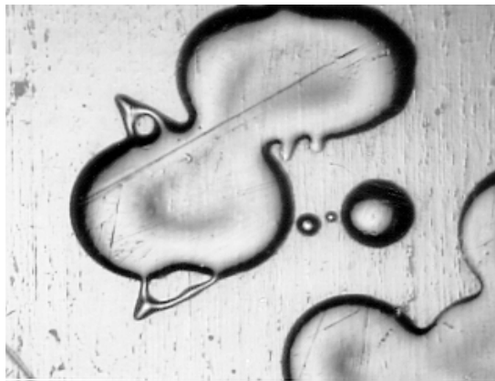
Figure 6—Unacceptable Ink-jet Markings
