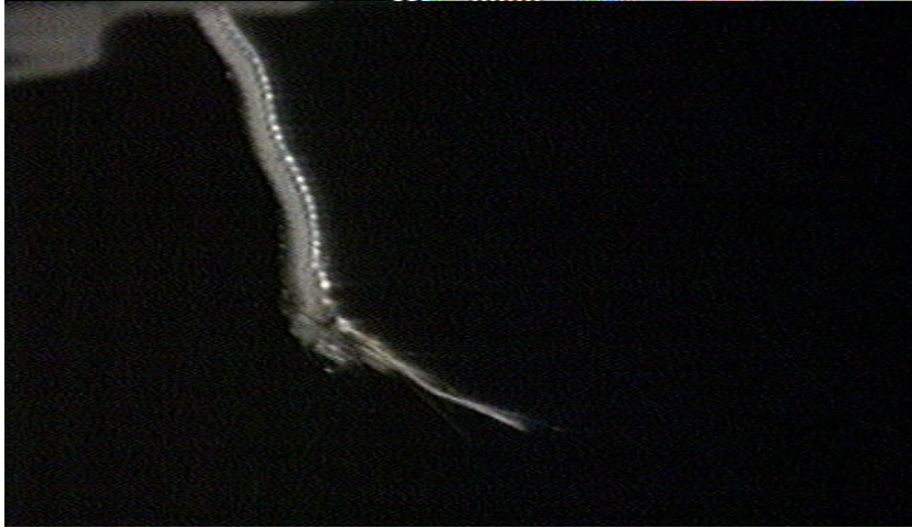
Figure 8—The End of the Remaining TSS-1R Tether (Ferguson and Hillard, 2003)
