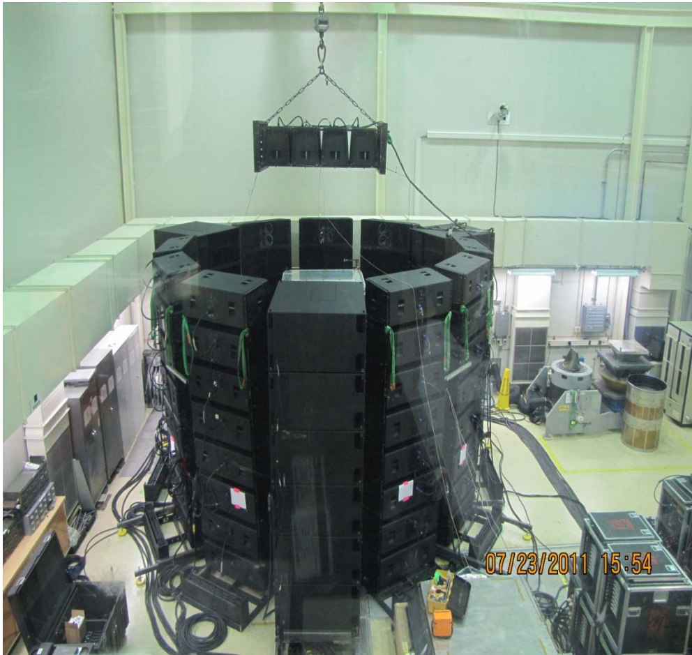
Figure 3—Current Speaker System Arrangements (Maahs, 2010, 2012)
