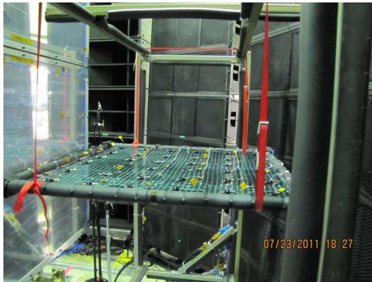
Figure 8—A Microphone Array Used to Obtain Spatial Mapping of the SPL in Various Slices of the Test Field
