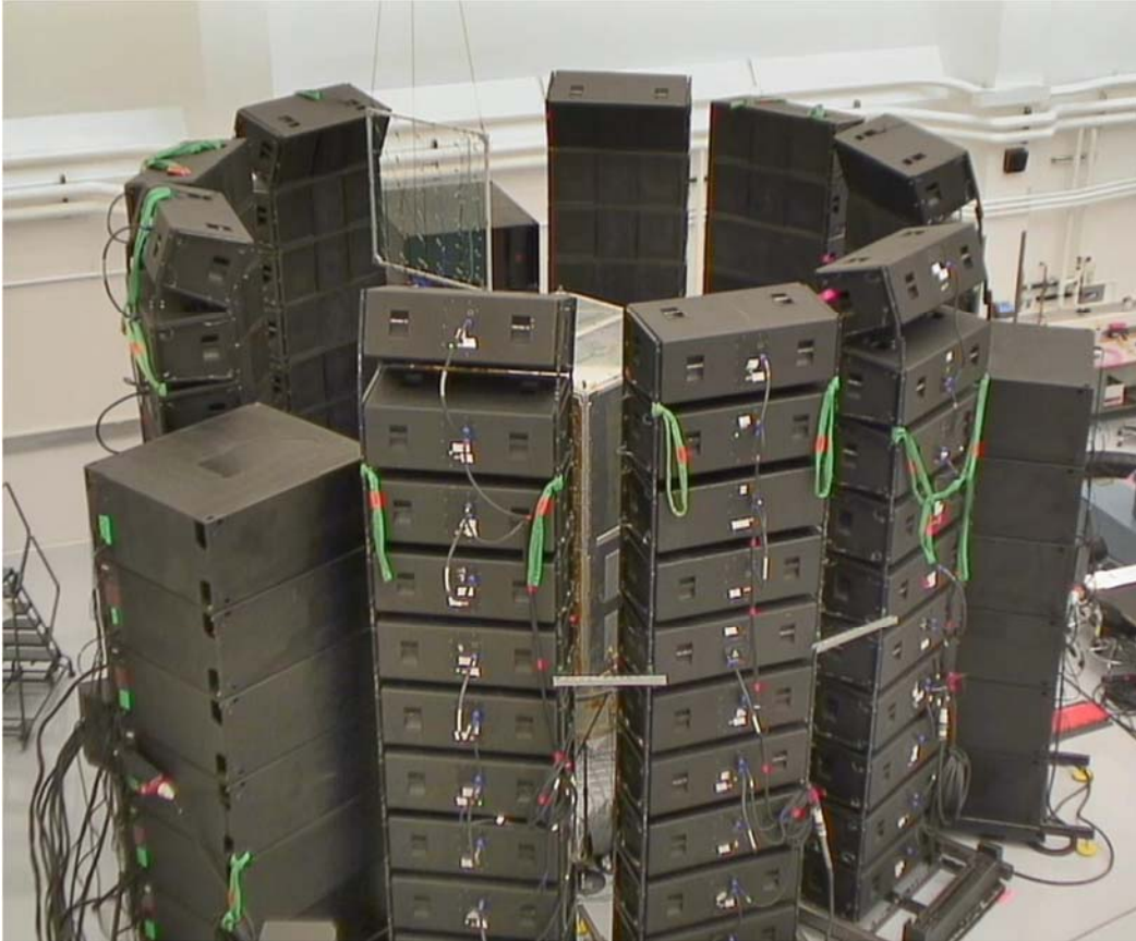
Figure 6—Example of a Test Setup for a Loudspeaker Array Diameter of 4.9 m (16 ft) (Maahs, 2010)
