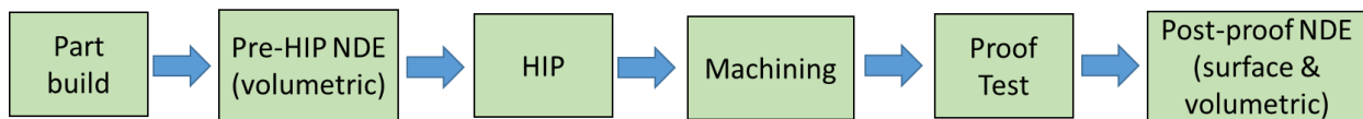
Figure 3—Typical Class A Fracture Critical Hardware Acceptance Steps Highlighting Placement of NDE Steps
