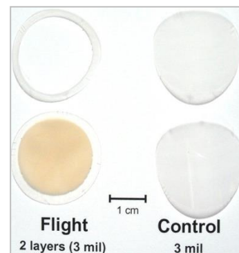
Post-flight photograph of individual sample layers. Layers were separated for weighing. (Mass loss Situation 2)
