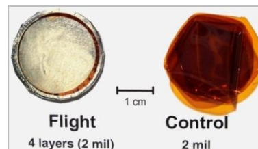
Post-flight photograph of stacked sample layers. Sample layers could not be separated for weighing. (Mass loss Situation 2)
