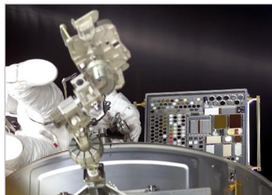
(b) Securing the PEC in the Opened Position, Exposing the Samples to Space
