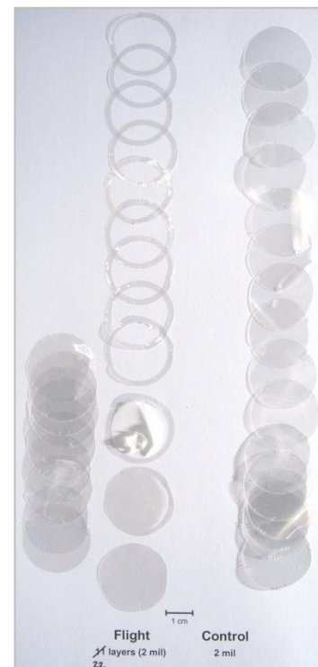
Post-flight photograph of individual sample layers. Layers were separated for weighing.
