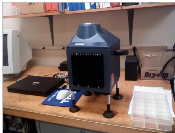
Figure 59—SOC 400T Reflectometer
