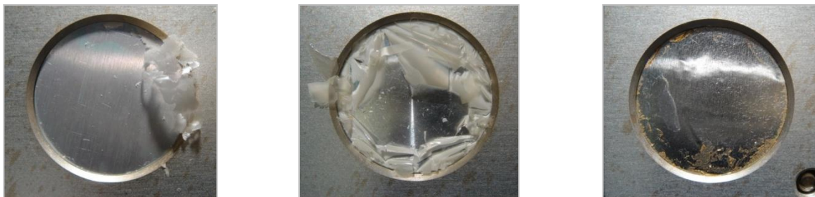
(a) Partially Eroded PE (2-E5-9) (b) Partially Eroded PMMA (2-E5-16) (c) Completely Eroded PBI (2-E5-35)
