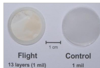
Post-flight photograph of stacked sample layers
