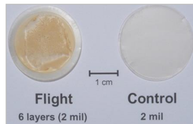
Post-flight photograph of stacked sample layers
