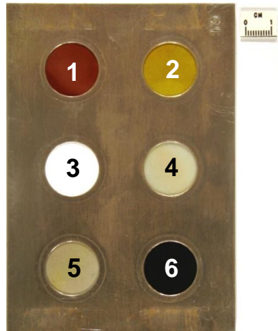
Figure 45—Sample Holder with Six Polymer Samples
