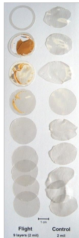
Post-flight photograph of individual sample layers. Layers were separated for weighing post flight. (Mass loss Situation 1)
