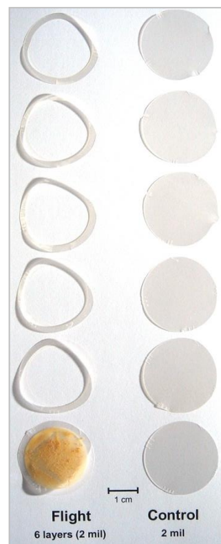
Post-flight photograph of individual sample layers. Layers were separated for weighing. (Mass loss Situation 2)
