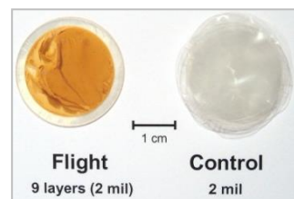
Post-flight photograph of stacked sample layers
