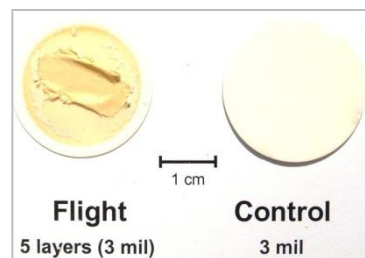
Post-flight photograph of stacked sample layers. Sample layers could not be separated for weighing. (Mass loss Situation 3)
