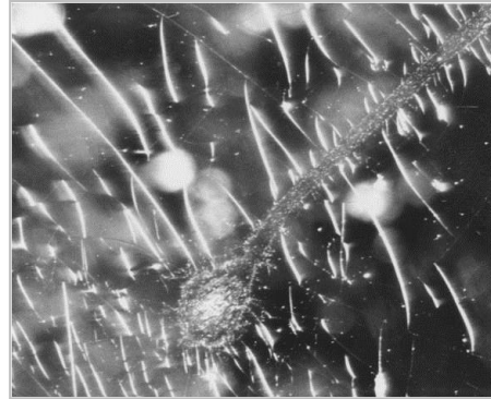
(b) Post-Flight with Mud-Tile Cracking Observed
