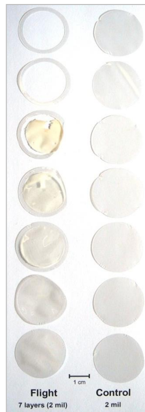
Post-flight photograph of flight and control sample individual sample layers. Layers were separated for weighing post-flight. (Mass loss Situation 2)
