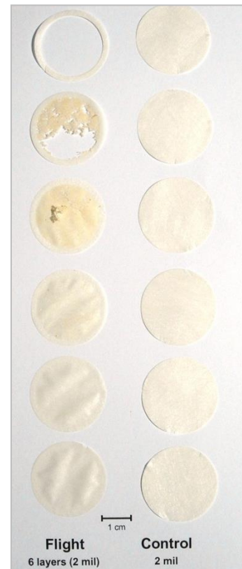
Post-flight photograph of individual sample layers. Layers were separated for weighing. (Mass loss Situation 2)
