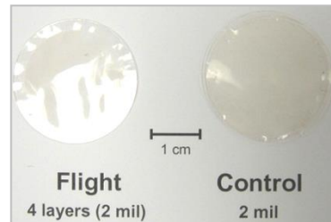
Post-flight photograph of stacked sample layers
