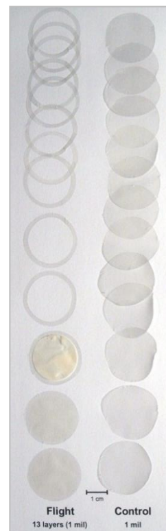
Post-flight photograph of individual sample layers. Layers were separated for weighing. (Mass loss Situation 2)
