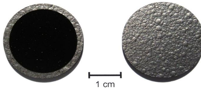
(a) Flight Sample (2-E5-25) (b) Control Sample
