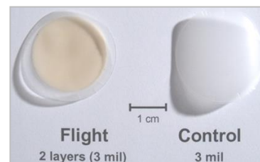
Post-flight photograph of stacked sample layers
