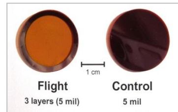
Post-flight photograph of stacked sample layers
