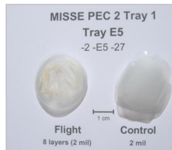
Post-flight photograph of stacked sample layers
