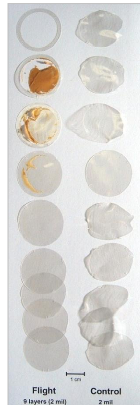
Post-flight photograph of individual sample layers. Layers were separated for weighing post flight. (Mass loss Situation 1)
