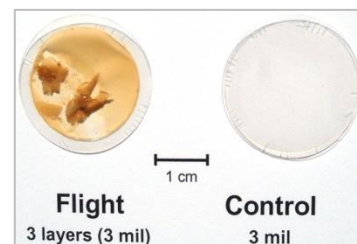
Post-flight photograph of stacked sample layers. Sample layers could not be separated for weighing. (Mass loss Situation 3)
