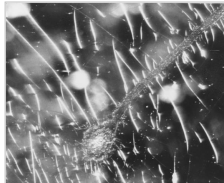
(b) Post-Flight with Mud-Tile Cracking Observed
