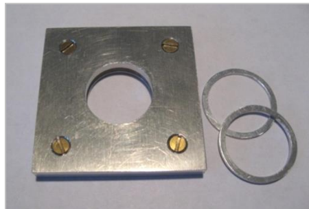
Figure 57—Sample Holder for Optical and Thermal Measurements
