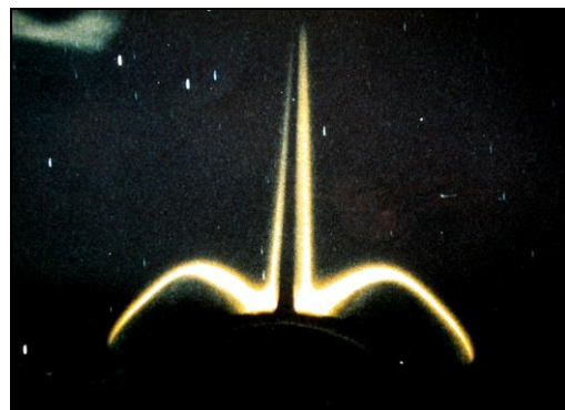
(b) Time-Lapsed Image Taken at Night with “Shuttle Glow” Visible
