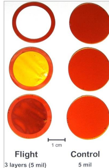
Post-flight photograph of individual sample layers. Layers were separated for weighing. (Mass loss Situation 2)
