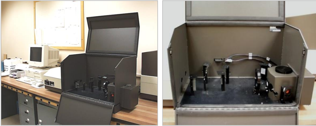
Figure 57—Perkin Elmer Lambda 19 Spectrophotometer with Closeup of Integrating Sphere
