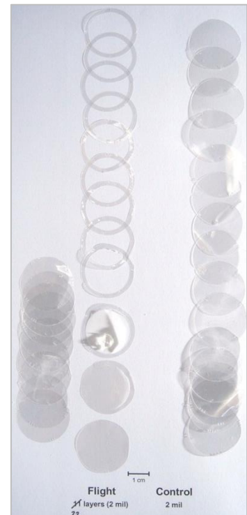
Post-flight photograph of individual sample layers. Layers were separated for weighing. (Mass loss Situation 1)
