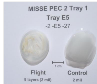
Post-flight photograph of stacked sample layers
