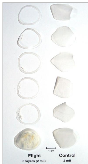
Post-flight photograph of individual sample layers (layers 6, 7, and 8 are together. Layers could be separated but were weighed together because of fragile pieces. (Mass loss Situation 3)
