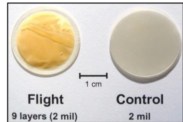
Post-flight photograph of flight and control stacked sample layers. Sample layers could not be separated for weighing. (Mass loss Situation 3)
