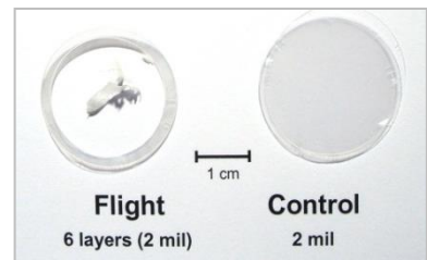
Post-flight photograph of stacked sample layers
