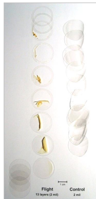
Post-flight photograph of individual sample layers. Layers were separated for weighing. (Mass loss Situation 2)
