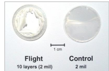
Post-flight photograph of stacked sample layers. Layers could not be separated for weighing post flight. (Mass loss Situation 3)
