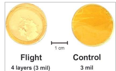
Post-flight photograph of stacked sample layers. Sample layers could not be separated for weighing. (Mass loss Situation 3)
