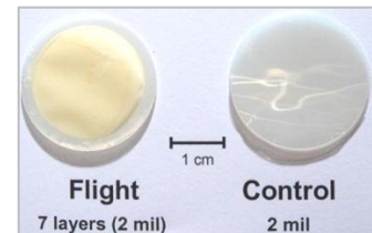
Post-flight photograph of stacked sample layers
