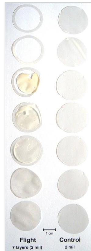
Post-flight photograph of flight and control sample individual sample layers. Layers were separated for weighing post-flight. (Mass loss Situation 2)
