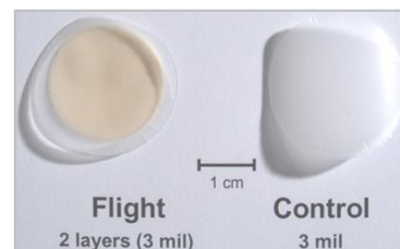
Post-flight photograph of stacked sample layers
