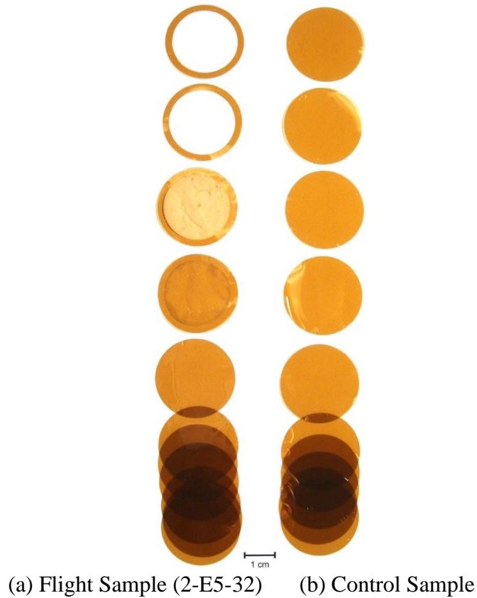
Figure 37—Post-Flight Photograph of PI (Upilex-S®) with Layers Separated (11 Layers, each 0.025 cm thick)
