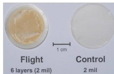
Post-flight photograph of stacked sample layers
