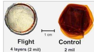
Post-flight photograph of stacked sample layers. Sample layers could not be separated for weighing. (Mass loss Situation 2)
