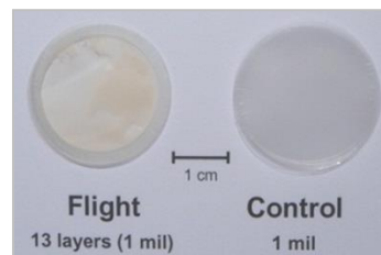
Post-flight photograph of stacked sample layers
