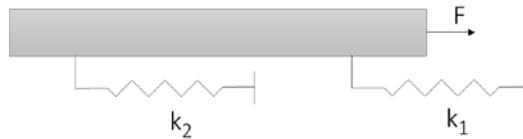
Figure 22a—Simplified Two-Bolt Plasticity Model
