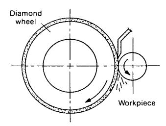
Figure 3—Outside Diameter Cylindrical Grinding for Machining Cylindrical Tension/Compression Rods
