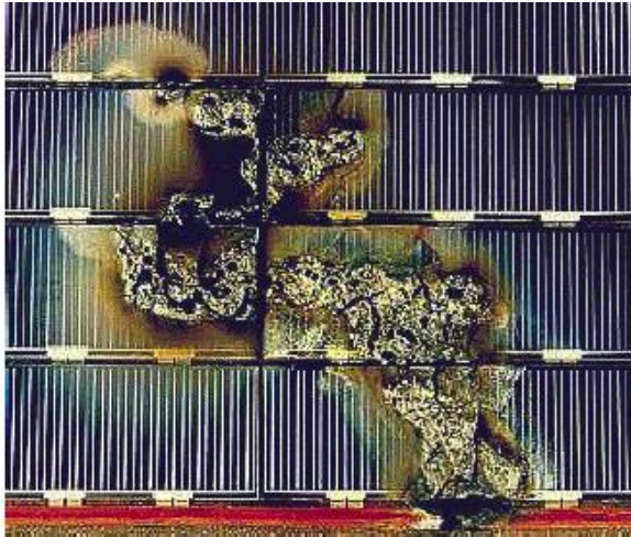
(a) Failure caused by in-flight ESD arcing
