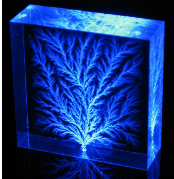
Figure 7—Example of Lichtenberg Figure by ESD
