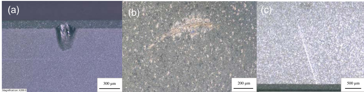
Figure 4—Damage to a Ceramic Crystal: (a) Tool Chip on Bevel; (b) Micrometer Edge Damage; (c) Tool Scratch
