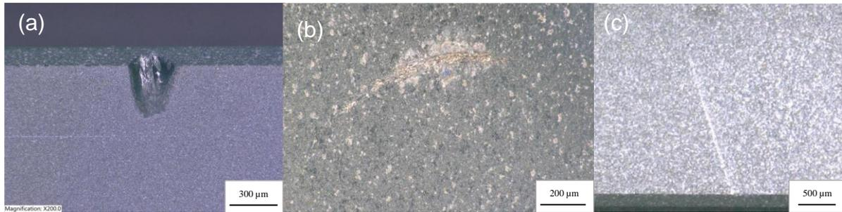
**Figure 4—Damage to a Ceramic Crystal: (a) Tool Chip on Bevel; (b) Micrometer Edge Damage; (c) Tool Scratch**
