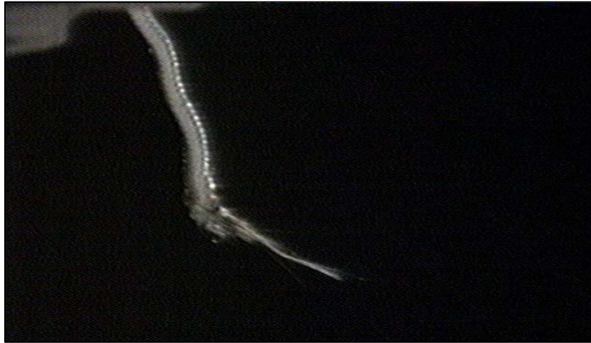
Figure 11—The End of the Remaining TSS-1R Tether (Ferguson and Hillard, 2003)
