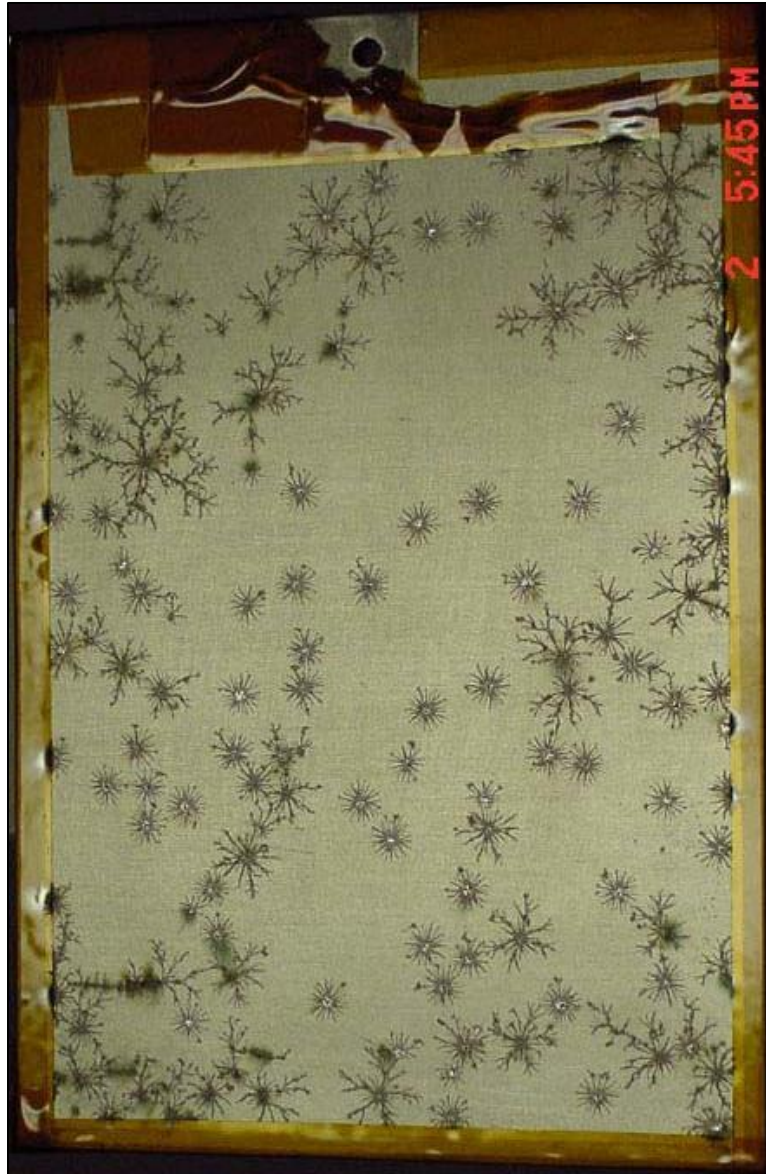
Figure 10—Anodized Aluminum Plate after Repeated Dielectric Breakdown Arcing (Schneider, et al., 2002b)
