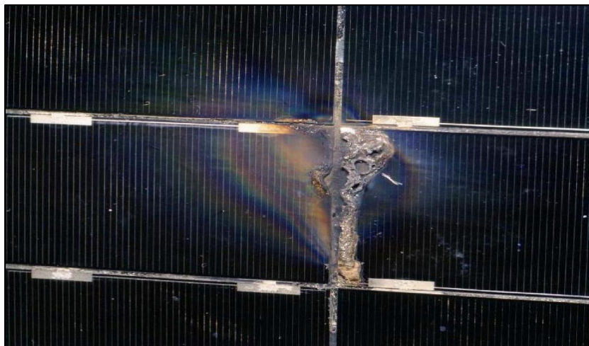
Figure 9—Arc Site of Sustained Arc on EOS-AM1 Sample Array. Cells are 2x4 cm. (Ferguson and Hillard, 2003)
