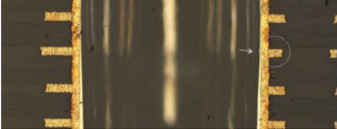
Figure 1 – Plated through hole microsection
